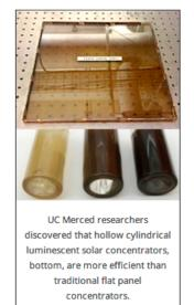
The research team showed the problem can be addressed by changing the shape of the concentrator. They discovered a hollow cylindrical solar concentrator is a better design compared with a flat concentrator or a solid cylinder concentrator. The hollow cylinders absorb more sunlight while having lower self-absorption losses.
